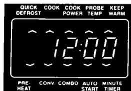
When you are not using the convection microwave oven, this is an accurate digital clock. When you are using the oven, it displays time settings, indicator lights and shows what number pads you touched.
